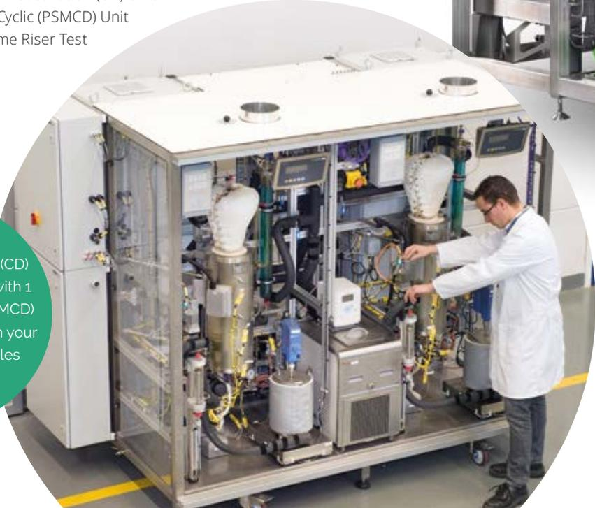
A Cyclic Deactivation (CD) unit can be supplied with 1 (CD), 2 (2-MCD) or 4 (4-MCD) reactors, depending on your need for E-cat samples
