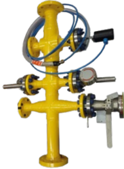
Example of a pipe spool for a Condensate Sampling System containing a Static Mixer, a manual sample take off, an automatic isokinetic grab sampler connection, a dual density measurement probe, a dissolved water in oil probe and a thermowell / PT100 connection.
