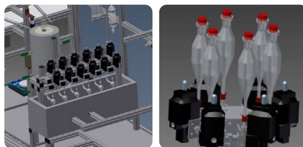
The SCT-RT unit can be outfitted with an automatic catalyst loading hopper and condenser system. The operator can program six runs. The six catalyst hoppers are connected to a general catalyst unloading system. The six condenser system is designed in such way that the unit K-factor will not depend on the condenser selection.
